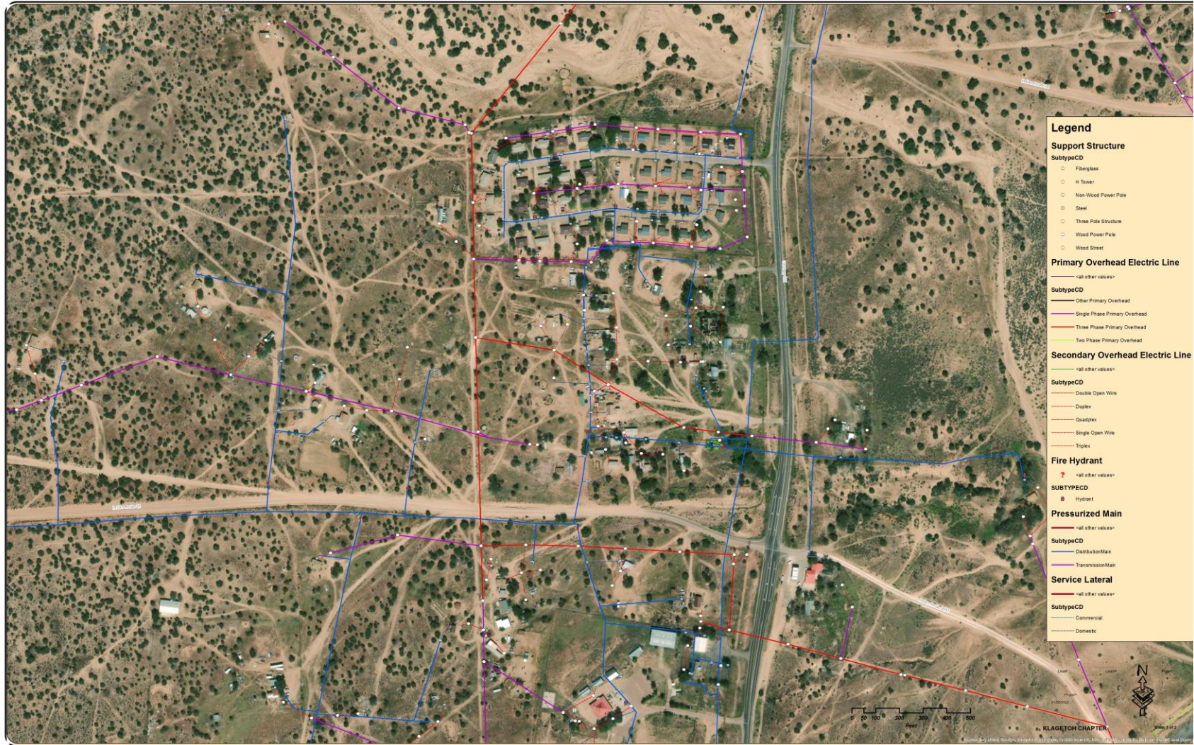
Photo 18. Central. This photo depicts the NTUA utility infrastructure for the NHA neighborhood, BIA Compound, and Chapter.
